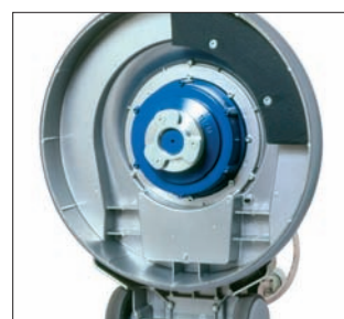
Attacco disco trascinatore e spazzole Mount for drive board and brushes
